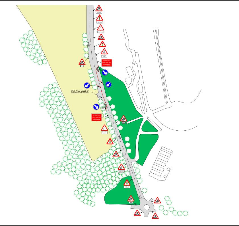
Traffic Signal Head Timings Head 1 Green 45 sec Red 20 sec Head 2 Green 45 sec Red 20 sec Key Chart: ----Road Sign Cones . Traffic Signal Head . Customer: Alun Griffiths Job Reference: Location: A466, Chepstow Date: 17.08.11 Decription: 2 Way Lights Amberon TM Ltd Tel: 07584993589 Fax: 01792 774590 Produced By: D.Green Drawing Ref: DG/170811.183/S The Deaving is ubject to Capyright and remains the property of J Amberon
